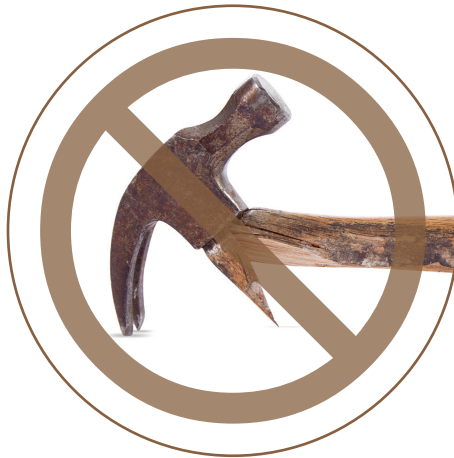
Using a hammer with a cracked handle
