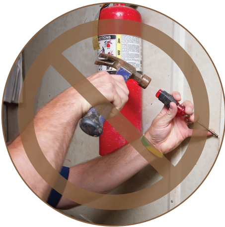
Using a screwdriver as a chisel
